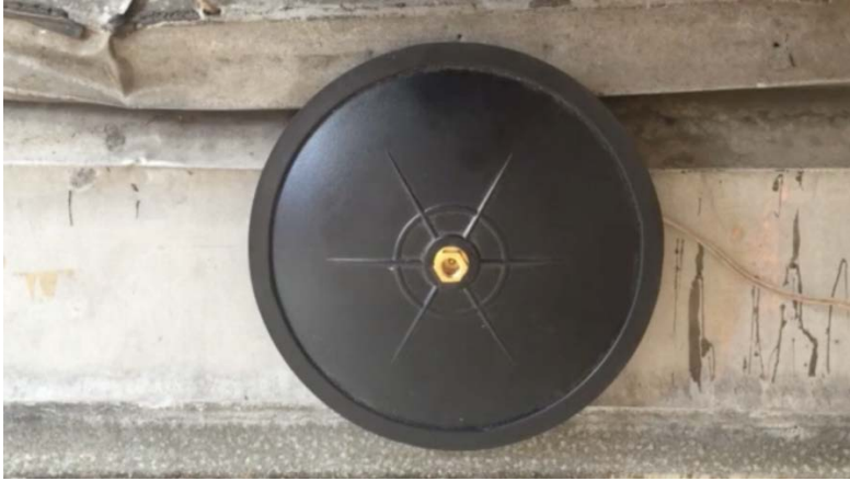
Figure 19. Transducer on corrugated metal
